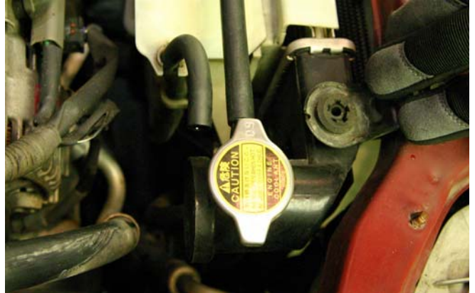
Okay to use conventional radiator pressure cap
