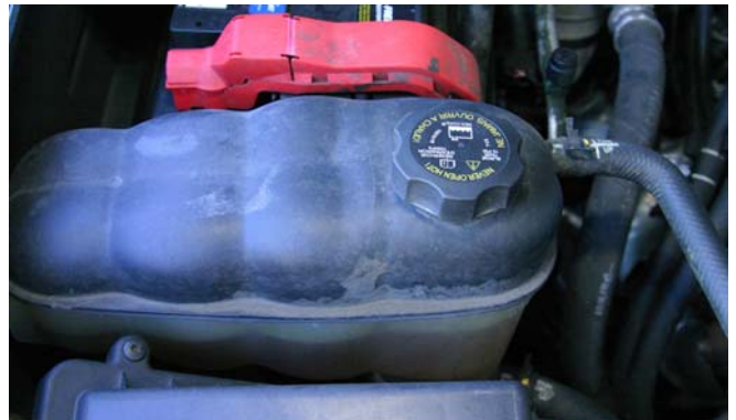
Okay to use coolant purge bottle (note pressure cap)
