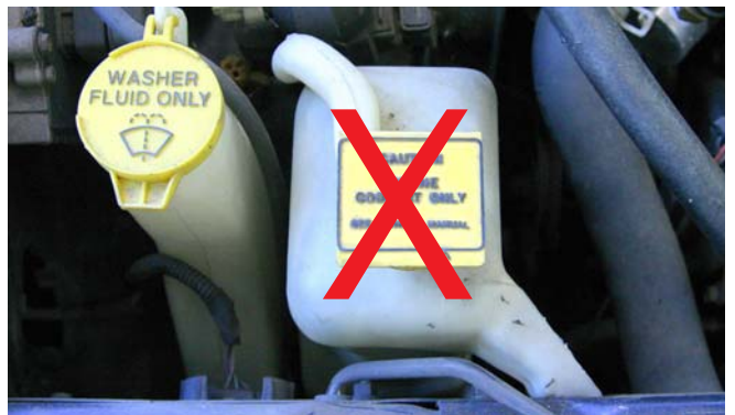
Do not use coolant overflow bottle
